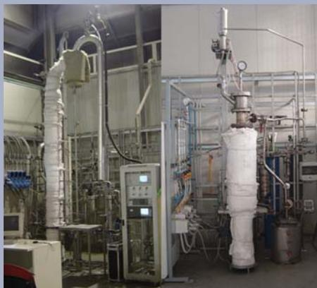
The laboratory scale fluidized bed gasifiers
