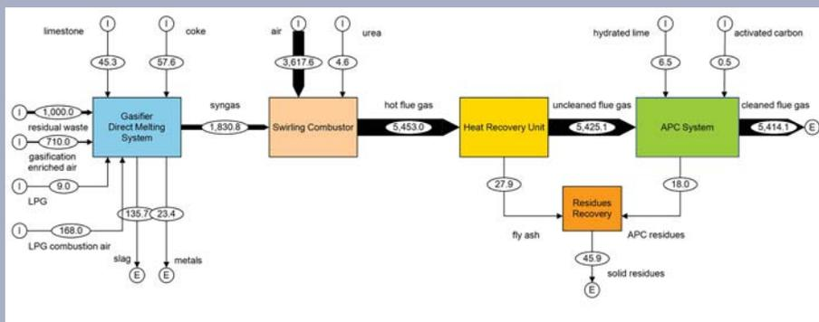
An example of MFA applied to a gasification-based thermal treatment
