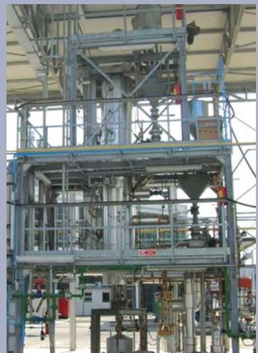
The pilot scale fluidized bed gasifier
