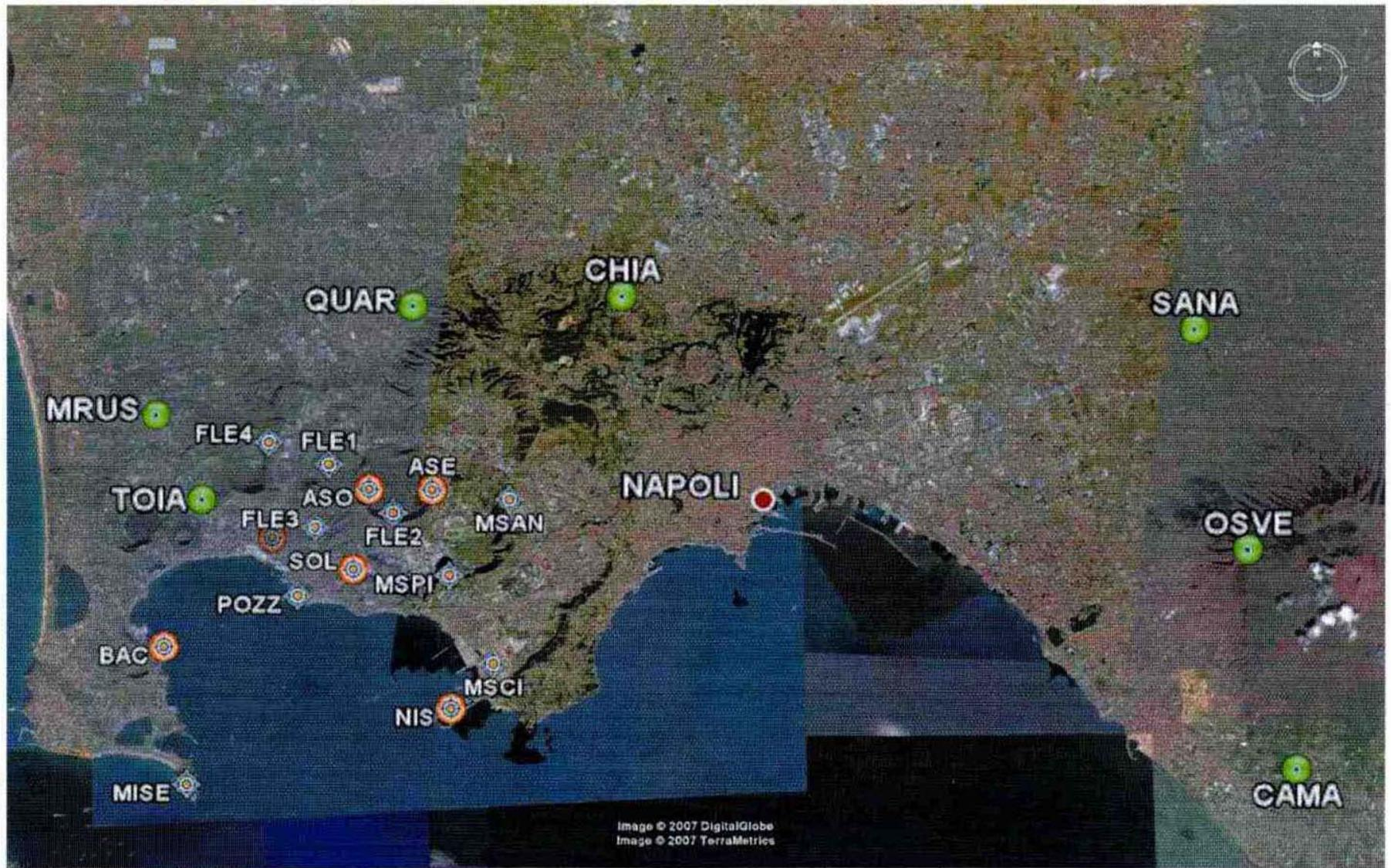
Fig. Green dots are the locations of the borehole dilatometers and surface broadband seismometers around Mount Vesuvius and Campi Flegrei. Only a borehole seismometer was installed at site QUAR. Orange circles indicate the permanent network, and small white circles indicate the borehole seismometer network currently under installation. Google Earth imagery © Google Inc., Digital Globe, Terra Metrics, Europa Technologies. Used with permission.
