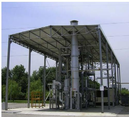
Fig. 3. Pilot-scale Bubbling Fluidized Bed Gasifier (BFBG), consists of the reactor having an ID of 0.381 m and a total height of 5.90 m, a high efficiency cyclone, a wet scrubber and a flare.
