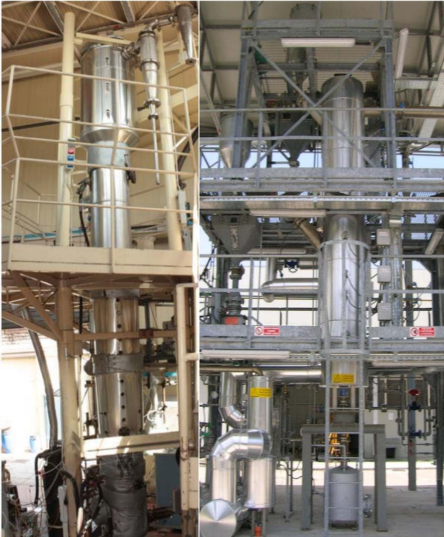
Figure 1. Photos of the two pilot-scale BFB reactors, combustion-based (left) and gasification-based (right).
